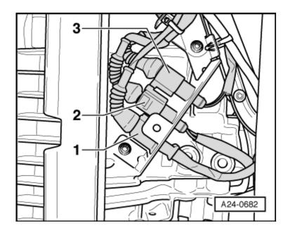
Remove oxygen sensor -arrow- using tool from Ring Spanner 7 piece set -3337-.
